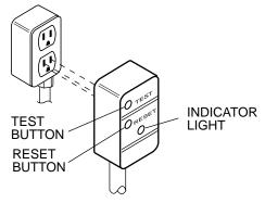
1. The spa is supplied with a 15 foot line cord which terminates with an integral GFCI plug. Locate the spa near enough to a weather protected outlet, but no closer than 10 feet. DO NOT USE AN EXTENSION CORD! Using an extension cord is hazardous and will decrease the amount of power to the unit, causing slow heating, poor whirlpool performance, or system malfunction.
